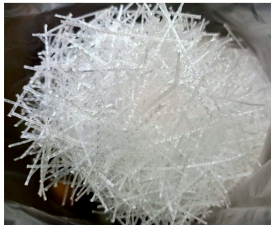
Figure 1. Structural macro synthetic polypropylene fibers.
