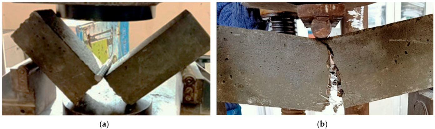
Figure 10. Cracking mechanism of concrete specimens under flexural strength test: (a) PCC (b) MSFRC.
