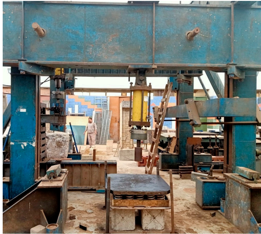
Figure 4. Concrete slab loading frame.
